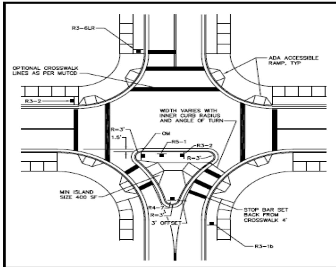
*Forced turn islands* will have clear widths sufficient for single-unit trucks (or buses if a transit route) to make turns at treated intersections without encroaching into opposing lanes. In addition, islands will be sharply angled toward the right on the approach to discourage wrong-way movement.
