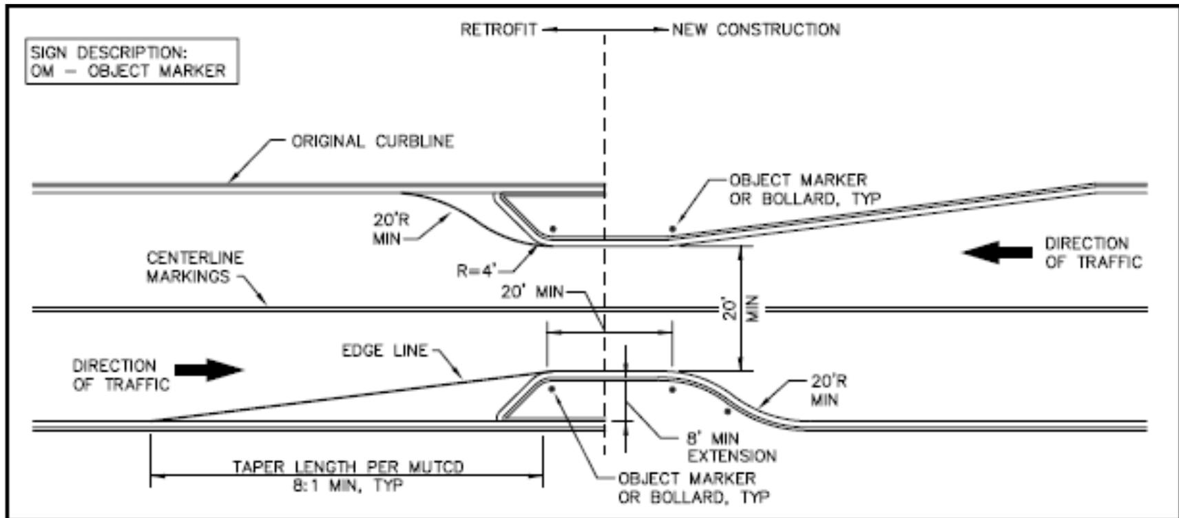
The typical two-lane *choker* is 25 feet from curb face to curb face. It has a minimum constricted length of 20 feet in the direction of travel, the length of a passenger car. The constricted length is kept short to avoid blocking driveways and displacing curbside parking.
