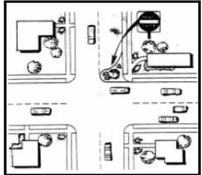
*Half street closures* are barriers that block travel in one direction for a short distance on otherwise two-way streets. They are also sometimes called *partial closures* or *one-way closures*. When two half closures are placed across from one another at an intersection, the result is a *semi-diverter* that blocks through movement on a cross street.
