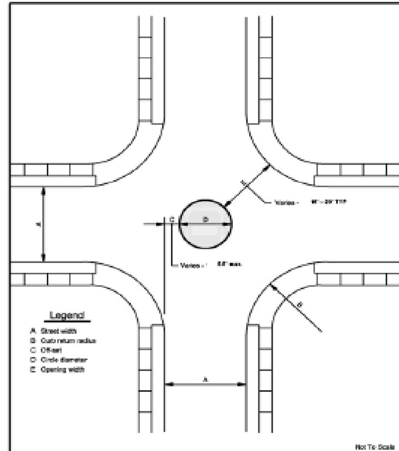
Most *traffic circles* have circular center islands and circular perimeters formed by the intersection corners. Where intersecting streets differ significantly in width, the center island may be elongated to better fit the intersection. An elongated circle consists of half-circles with tangent sections between them. Most traffic circles are deployed at four-way intersections, for this is where the greatest safety benefits accrue.
