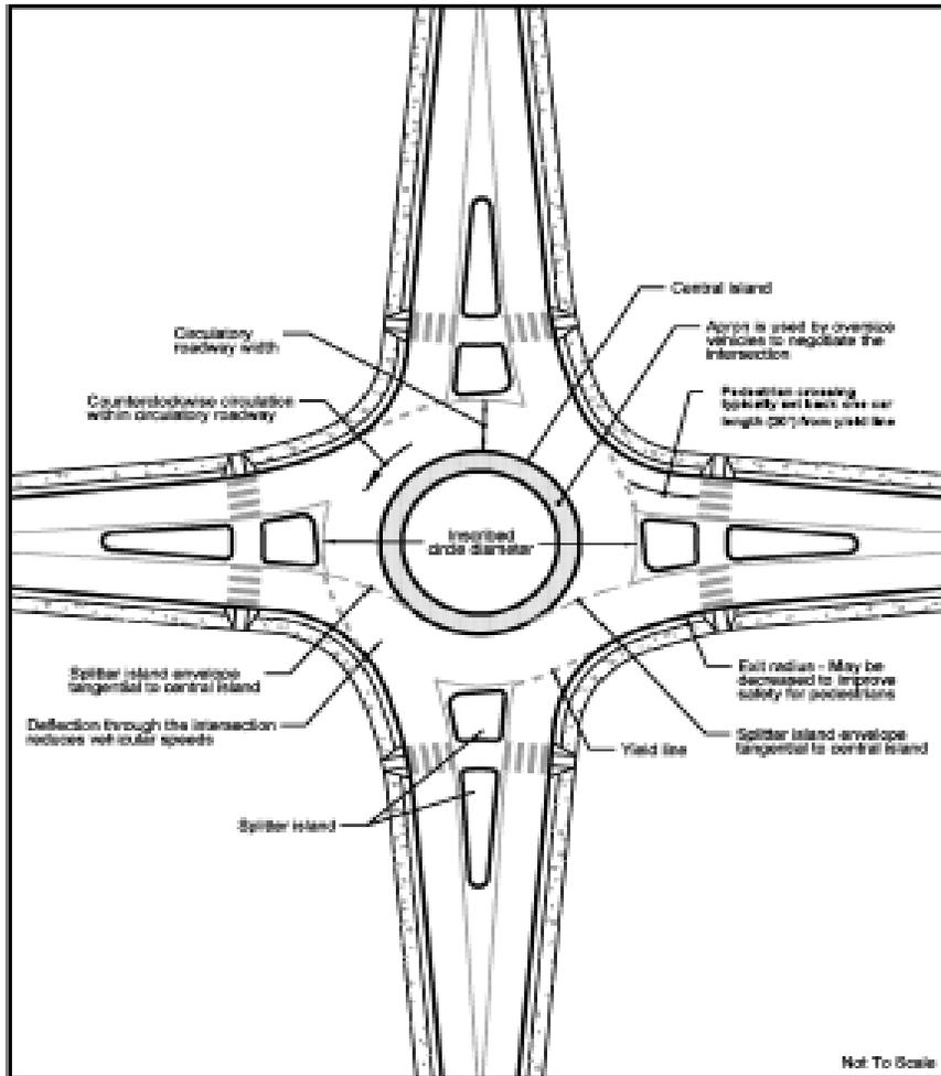
*Roundabouts* are distinguished from traffic circles by larger radii, correspondingly higher design speeds and capacities, and splitter islands on all approaches to slow traffic and discourage wrong-way movements.
