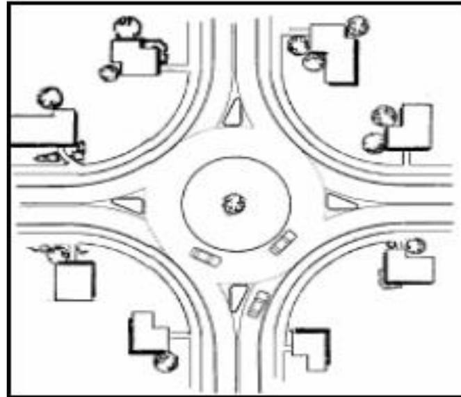
*Roundabouts*, similar to mini traffic circles in that traffic circulates around center islands, are used at higher volume intersections to allocate ROW among competing movements. Roundabouts in the U.S. are found primarily on arterial and collector streets, often substituting for traffic signals or all-way stops. They are larger than mini traffic circles, are designed for higher speeds, and have raised splitter islands to channel approaching traffic to the right.
