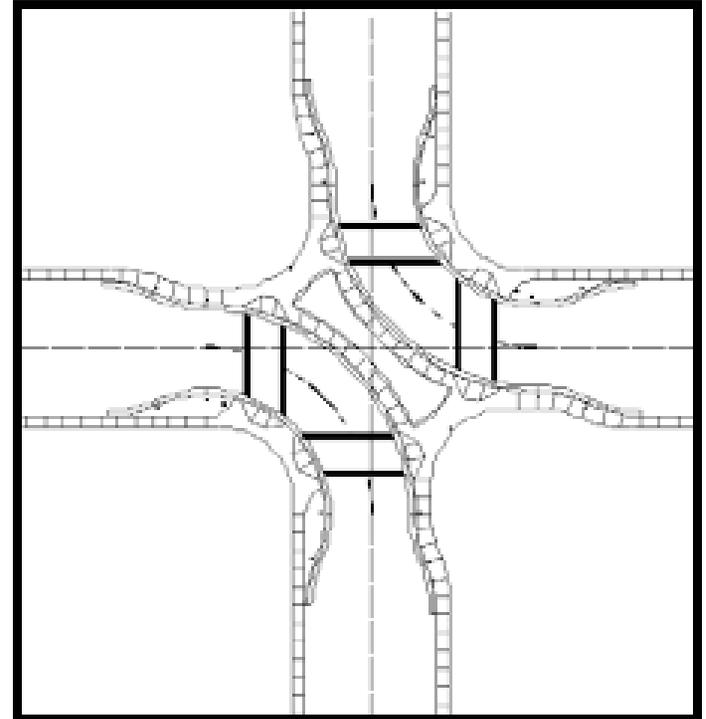
*Diagonal diverters* are barriers placed diagonally across an intersection blocking through movement. They are also called *full diverters* and *diagonal road closures*.
